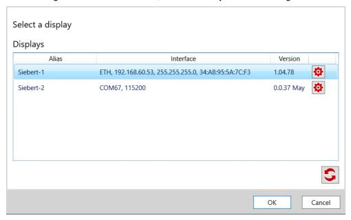
The search process of the TextLine One editor uses UDP broadcasts for searching. This means that displays are also found which are in a different network than the PC. However, searching across router boundaries is not possible due to network technical reasons.
